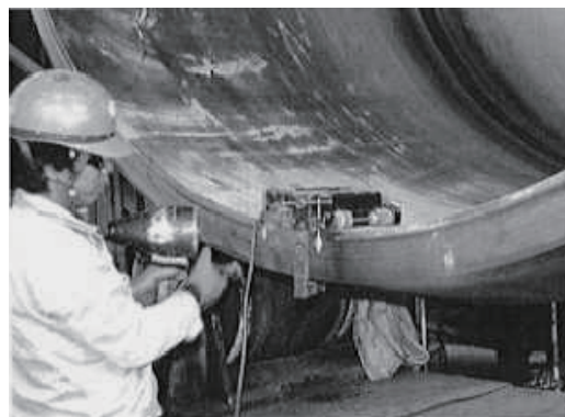
Photo 4.1 — Magnetic particle testing of the bevel surface of a welding joint with a heavy section
