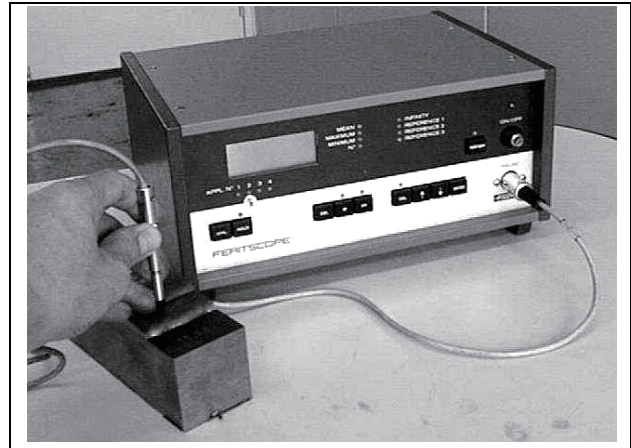
Photo 2.4 — Feritscope measures the voltage induced in the probe coil according to the ferrite content. This instrument is suitable for use at site because the probe is small enough to put on a small area of weld metal.
